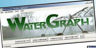
The WATERMARK Monitor is user-programmed for the individual characteristics of the site being monitored using WaterGraph Software WG3 for 900 Series Monitors.
